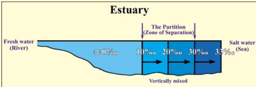
**Figure 14:** Longitudinal section showing salinity (parts per thousand ‰) in an estuary. We can see here the partition (zone of separation) between the fresh and the salt water. (*Introductory Oceanography*, Thurman, p. 301, with a slight enhancement.)
